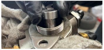
**Step 22** Insert the new piston into the HPFP assembly.
