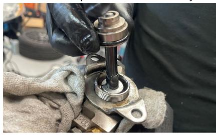
**Step 23**Replace the upper sleeve over the piston.
