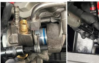
**Step 28** Reconnect the hardline to the fuel pump.
