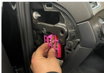
**Step 3**Locate the fuel pump fuse and remove it.
